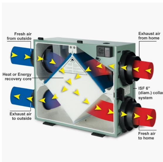
**How does it work?** Clean, fresh air is pulled into the building from outside, but before it is circulated around the house, this fresh air is passed over a heat exchanger. At the same time, warm stale air extracted from kitchens and bathrooms is also fed through the same heat exchanger. This allows the energy (In the form of heat) to be passed from the 'old' air to the 'new' air.
